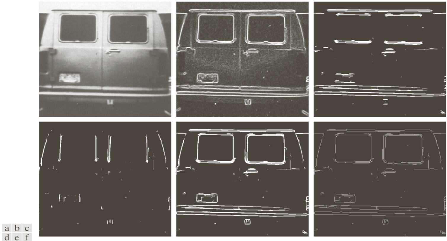
FIGURE 10.27 (a) A 534 \times 566 image of the rear of a vehicle. (b) Gradient magnitude image. (c) Horizontally connected edge pixels. (d) Vertically connected edge pixels. (e) The logical OR of the two preceding images. (f) Final result obtained using morphological thinning. (Original image courtesy of Perceptics Corporation.)
