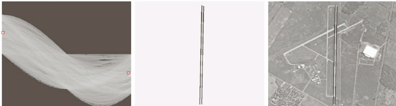
FIGURE 10.34 (a) A 502 \times 564 aerial image of an airport. (b) Edge image obtained using Canny's algorithm. (c) Hough parameter space (the boxes highlight the points associated with long vertical lines). (d) Lines in the image plane corresponding to the points highlighted by the boxes). (e) Lines superimposed on the original image.
