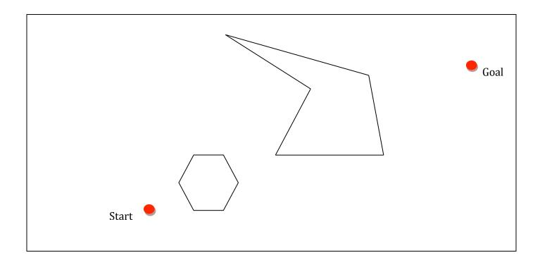
58) Draw the trajectory for the Bug2 path planning algorithm, starting position the robot goal the star. Consider a left turning robot.
