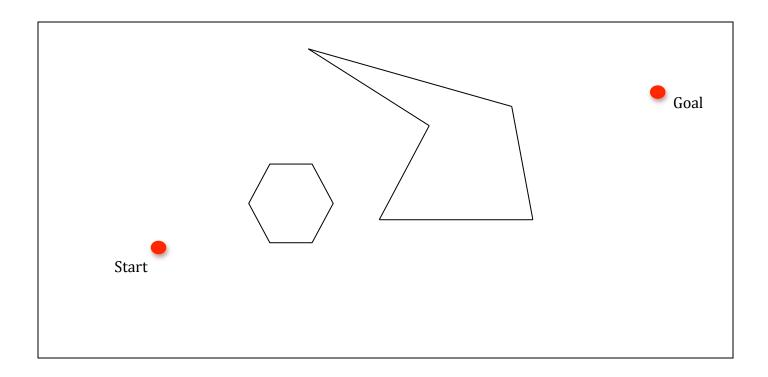
60) Use the grassfire transform to create the configuration space on the following world, dilating the obstacles by 2 pixel. Is the resulting space connected?
