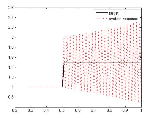
54)When a proportional controller tries to follow the step function (y=1: x<0.5; y=1.5: x>0.5) describe the possible causes for the response shown here:
