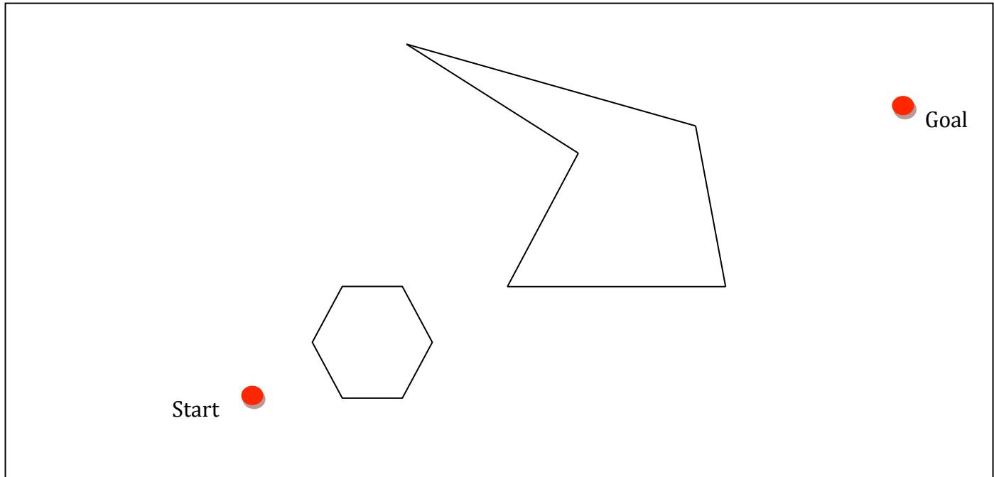
45) Draw the trajectory for the Bug2 path planning algorithm, starting position the robot goal the star. Consider a left turning robot.
