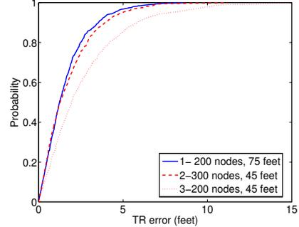
Fig. 5. Error CDF of the estimation of the jammer's transmission range.
