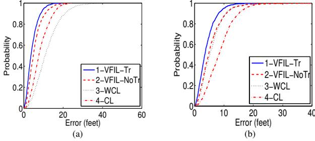
Fig. 3. Effects of the jammed area when  $N = 200$  and transmission range is 45 feet: (a) case 1 - only the jammed nodes that are within the transmission range of boundary nodes can send out ranging information; (b) case 2 - all the jammed nodes can send out ranging information.
