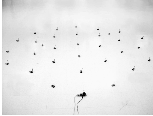
Fig. 6. Our Mica2 testbed consists of 30 nodes that are placed on the floor. Nodes are roughly separated from each other by 2.5 feet. The sink is located at the bottom of the figure, with a programming board attached to it.
