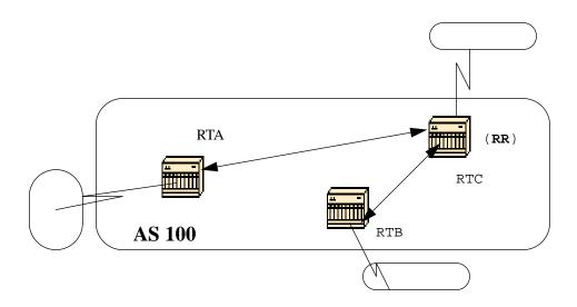
In normal cases, a full IBGP mesh should be maintained between RTA, RTB and RTC within AS100. By utilizing the route reflector concept, RTC could be elected as a RR and have a partial IBGP peering with RTA and RTB. Peering between RTA and RTB is not needed because RTC will be a route reflector for the updates coming from RTA and RTB.
