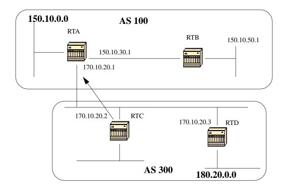
The following example shows how the nexthop will behave on a multiaccess network such as ethernet.
