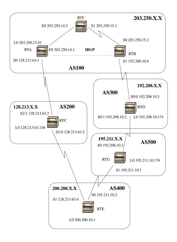
We will build the above configuration step by step and see what can go wrong along the way. Whenver you have an AS that is connected to two ISPs via EBGP, it is always good to run IBGP within your AS in order to have a better control of your routes. In this example we will run IBGP inside AS100 between RTA and RTB and we will run OSPF as an IGP.
