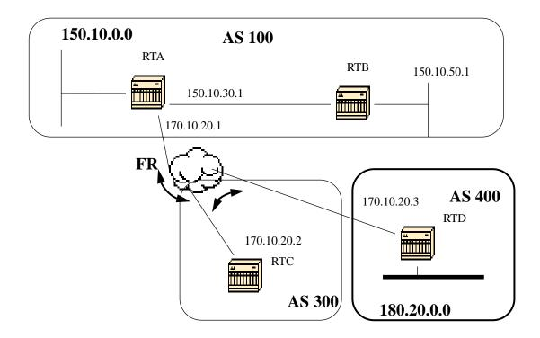
If the common media as you see in the shaded area above is a frame relay or any NBMA cloud then the exact behavior will occur as if we were connected via ethernet. RTC will advertise 180.20.0.0 to RTA with a next hop of 170.10.20.3.
