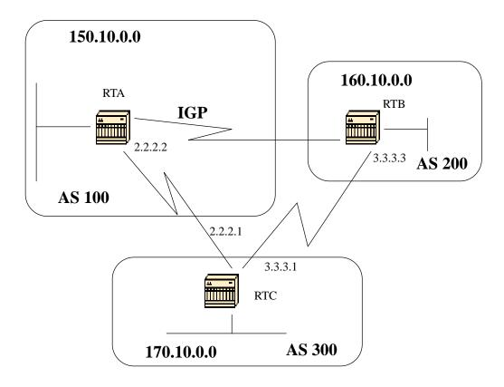
Consider the above diagram, RTA and RTC are running EBGP and RTB and RTC are running EBGP. RTA and RTB are running some kind of IGP (RIP, IGRP, etc.)
