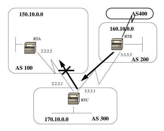
You can specify an access list on both incoming and outgoing updates based on the BGP autonomous system paths information. In the above figure we can block updates about 160.10.0.0 from going to AS100 by defining an access list on RTC that prevents any updates that have originated from AS 200 from being sent to AS100. To do this use the following statements.
