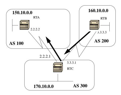
Request: Allow RTB to advertise the prefix 160.0.0.0 and suppress all the more specific routes. The problem here is that network 160.10.0.0 is local to AS200 i.e. AS200 is the originator of 160.10.0.0. You cannot have RTB generate a prefix for 160.0.0.0 without generating an entry for 160.10.0.0 even if you use the "aggregate summary-only" command because RTB is the originator of 160.10.0.0.
