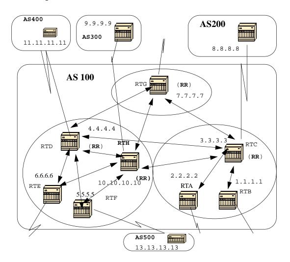
Usually, a cluster of clients will have a single RR. In this case, the cluster will be identified by the router-id of the RR. In order to increase redundancy and avoid single points of failure, a cluster might have more than one RR. All RRs in the same cluster need to be configured with a 4 byte cluster-id so that a RR can recognize updates from RRs in the same cluster.
