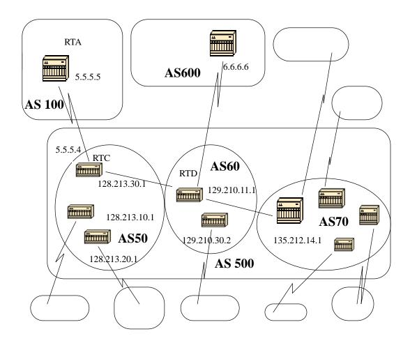
Let us assume that you have an autonomous system 500 consisting of nine BGP speakers (other non BGP speakers exist also, but we are only interested in the BGP speakers that have EBGP connections to other ASs). If you want to make a full IBGP mesh inside AS500 then you would need nine peer connections for each router, 8 IBGP peers and one EBGP peer to external ASs.
