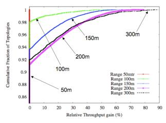
Figure 6: Two transmissions to different receivers: no gain from SIC in 90% of the cases.
