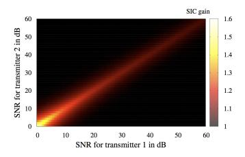
Figure 2: SIC capacity gains are not high in general but are larger when RSSs are smaller and similar.
