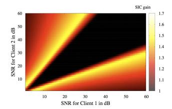
Figure 4: Two transmitters to the same receiver: SIC gains most when RSSs are such that the resulting bitrates are the same for both transmissions.
