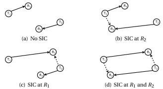
Figure 5: Two transmitters to different receivers: signal of interest (solid) and strong interference (dashed)
