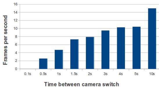
Figure 1: The resulting frame rate on a Samsung Galaxy Note with varying time between camera switches. Frequent switching reduces frame rate.
