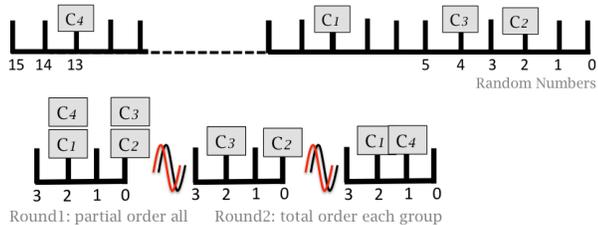
**Figure 1: Key observation behind hierarchical backoff: Top WiFi time-line shows an attempt to total-order all nodes, while we attempt to partial-order nodes (into groups) and then total order each smaller group.**
