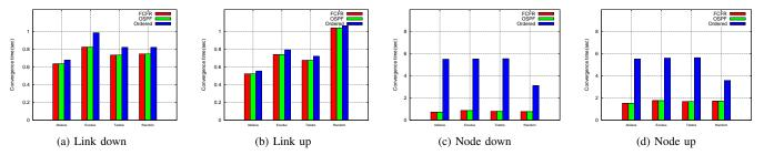
Fig. 3. Convergence time, as measured by the time at which all routers in the network have finished updating their forwarding tables after a network event. OSPF, FCFR, and SafeGuard (not shown) have identical convergence times, while ordered updates requires a longer convergence time.
