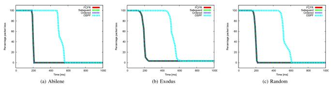
Fig. 6. Packet loss rates for a single link down event. Fast rerouting algorithms (i.e. FCFR, SafeGuard, and ordered updates) stop losing packets immediately after the failure is detected, while OSPF continues to lose packets until forwarding tables are updated.
