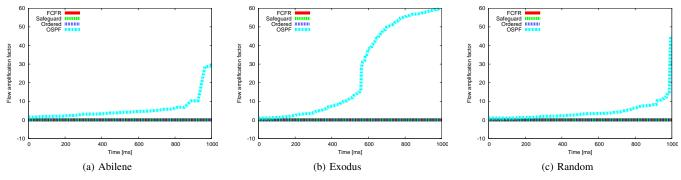
Fig. 5. Flow amplification factor for a single link down event. SafeGuard, ordered updates, and FCFR guarantee loop prevention during the convergence interval and therefore do not have flow amplification by definition. OSPF has routing loops during convergence, and thus a higher flow amplification factor.
