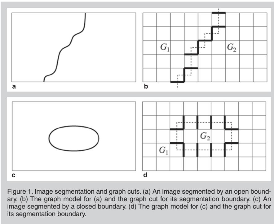
Figure 1. Image segmentation and graph cuts. (a) An image segmented by an open boundary. (b) The graph model for (a) and the graph cut for its segmentation boundary. (c) An image segmented by a closed boundary. (d) The graph model for (c) and the graph cut for its segmentation boundary.
