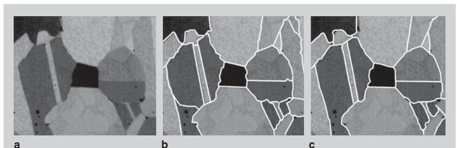
Figure 2. Segmentations on a (a) (cropped) Ni-based alloy image using (b) normalized cut and (c) ratio cut.
