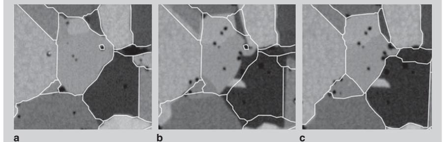
Figure 3. Segmentation of a (a) (cropped) Ni-based alloy image by optimal labeling. (a) Segmented grain boundaries in a template slice. (b) Grain boundaries in (a) copied to a new slice. (c) Segmented grain boundaries in this new slice after optimal labeling.
