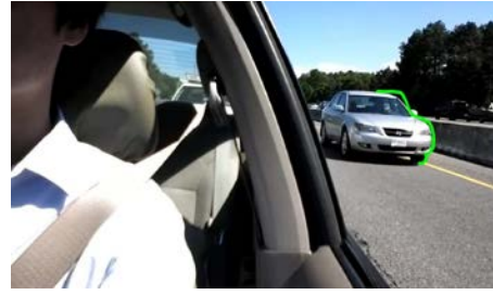
Fig. 4. Chamfer Matching of the template to a vehicle.
