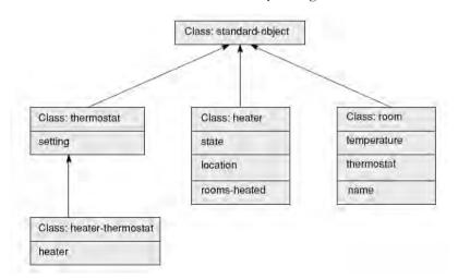
Figure 18.2. A class hierarchy for the room/heater/thermostat simulation.
