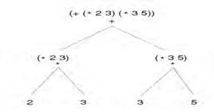
Figure 11.1. Tree representation of the evaluation of a simple Lisp function
