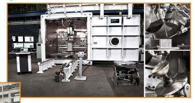
E-beam Additive Manufacturing System
