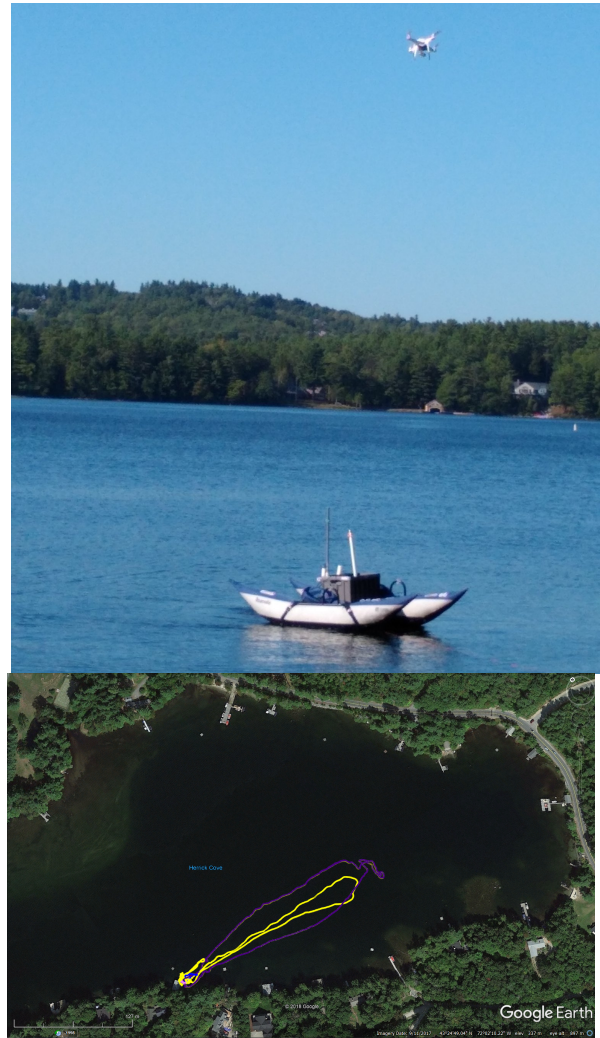
Fig. 3: Preliminary experiments with a boat and drone at Lake Sunapee, NH, in collaboration with the Lake Sunapee Protective Association, and a transect where traditional sampling (manual and buoy) is combined with a robot.
