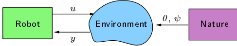
Fig. 1. As the robot interacts with its environment, an artificial decision maker nature generates disturbances.
