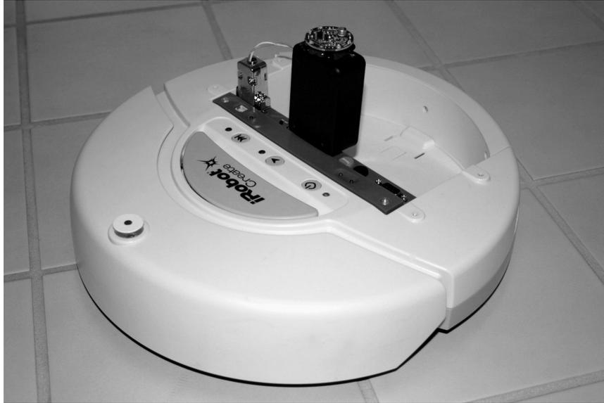
**Fig. 4.** An iRobot Create differential drive robot, equipped with a 4 infrared beacons and 4 infrared sensors. When deployed in pairs, such robots can track one another by sensing which quadrant contains the other robot.
