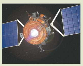
Figure A. Close-up of the Remote Agent, ion engine firing. (courtesy of NASA Ames/JPL)
