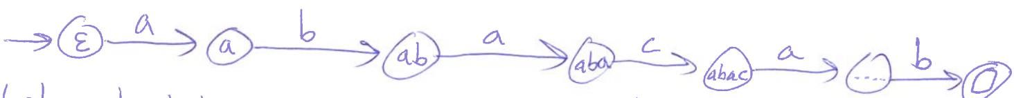
Label each state with a ~~label~~ the corresponding prefix of  $x$  by reading from the start state.
