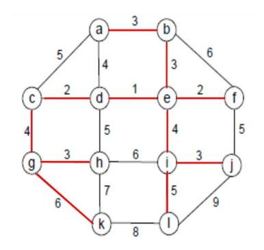
The MST consists of the edges ab, be, ed, dc, ef, cg, gh, ei, ij, il, and gk
