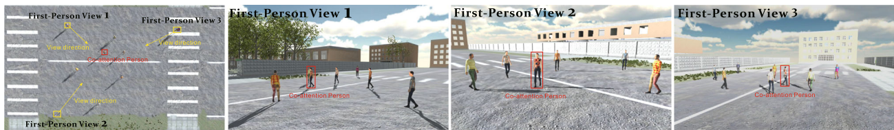
Fig. 13 An illustration of the co-attention human detection using complementary-view cameras with the relative view direction
