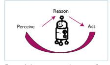
Figure 1.A common architecture for robot behavior. A robot with this PRA architecture would use its sensors to perceive its environment, reason about its perceptions, and then decide on an action.
