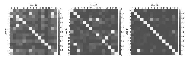
Figure 6: All users facing the glass: (a) Similarity scores from spatiograms; (b) Confidence scores from classification using wavelet features; (c) The effect of combining color with patterns.
