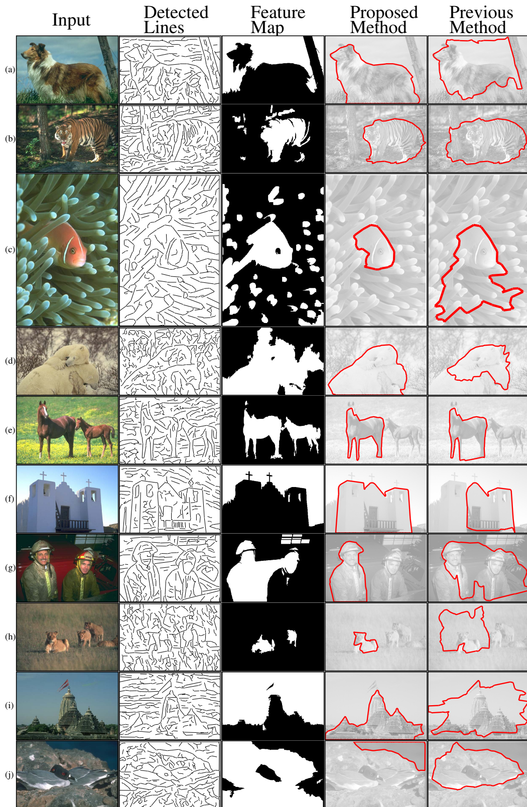
Figure 6. Results on 10 real images. From left to right, each column shows the original image, the segments produced by the edge detection and line approximation, the binary feature map, the result obtained by the proposed method, and the result obtained by a comparison method [22].
