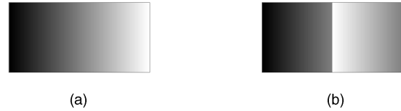
Fig. 5. An illustration of why pixel-intensity variance is ill-suited as a measure of segment homogeneity. The intensity of image (a) varies uniformly from 0, at the left, to 255, at the right. The intensity of image (b) varies uniformly from 0, at the left, to 128, in the center, then abruptly changes to 255, and finally varies uniformly from 255 to 129, at the right. While the sets of pixel intensities in these two images have the same statistical properties, (a) appears to contain a single segment, while (b) appears to contain two segments.
